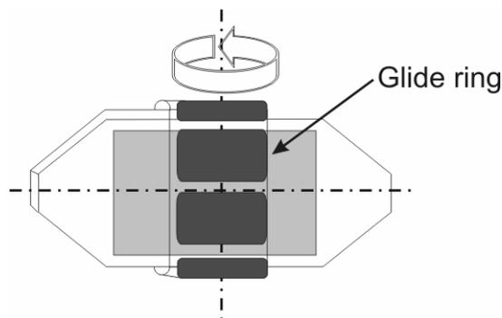
Figure 7: **KOMET** stirring bar with glide ring
