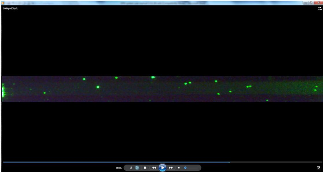
Example of an area of interest (1220 x 100 pixels) in a 170 ml mini swim tunnel. The area covers the complete length of the swim tunnel but not the entire height.
