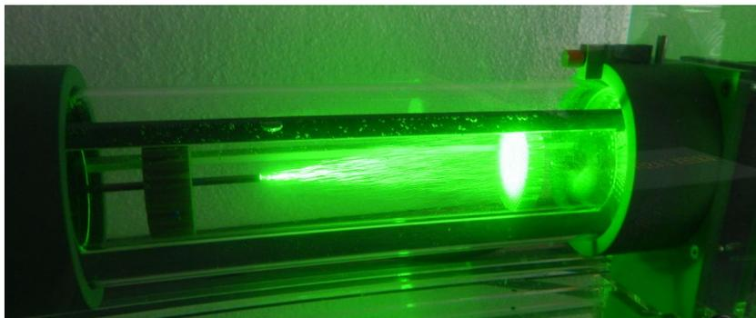
Example of laser placement in a 1.5 L Loligo® mini swim tunnel.
