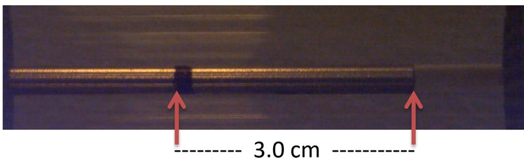
Remove the laser steel rod from the flow and place in the measuring position (see section 4.1) and continue with the flow velocity video recording.
