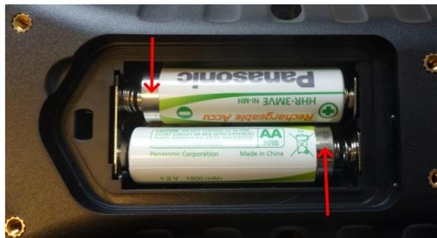
For rechargeable batteries (NiMH), there is the negative pole connected to the metal under the shrinking tube, for primary cells there is the positive pole. The golden contacts in the battery compartment check this and hence we can prevent that customers insert primary cells and the device tries to charge them (could result in leakage and hence in a damage of the electronics).
