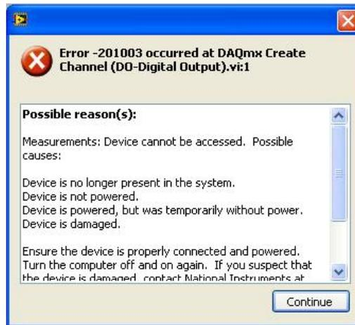
The error shown on Screen 23 occurs, when the NI-USB 6008/6009 DAQ card has no properly connection to the PC. This error can occur in 2 ways.
