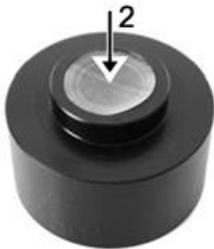
2) Place a new membrane on the base above the ring.
